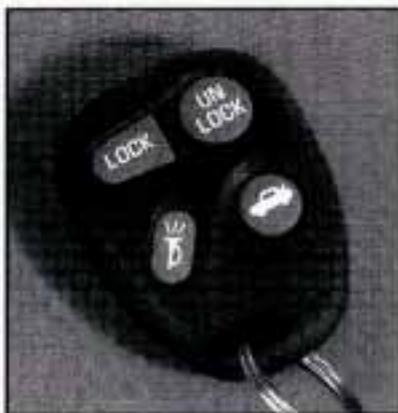
You can lock and unlock your doors or unlock your trunk from about 3 feet (1 m) up to 30 feet (9 m) away using the key chain transmitter supplied with your vehicle.
