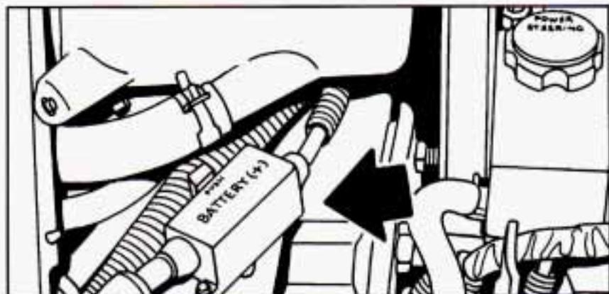
4. Open the hoods and locate the other vehicle's battery and the Aurora's remote positive (+) jump starting terminal in the box on the passenger side of the engine compartment. (Your Aurora's battery isn't under the hood.)
