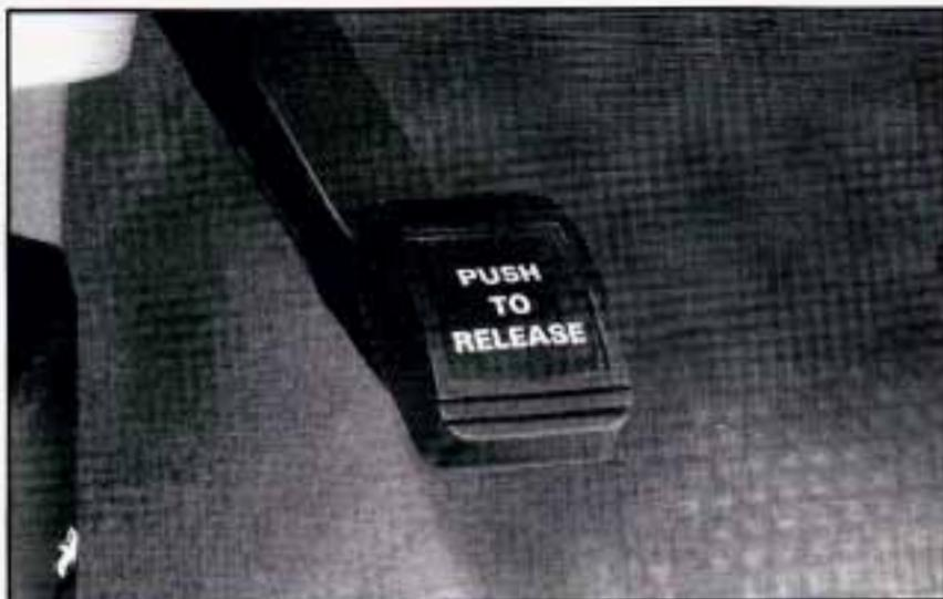
**Setting the parking brake:** Hold the regular brake pedal down with your right foot. Push down the parking brake pedal with your left foot. If the ignition is on, the parking brake indicator light will come on.
