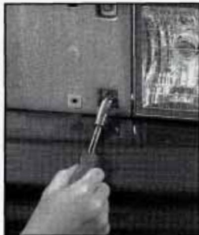
2. Use a 10 mm socket to remove the four bolts. There are two bolts on each side of the cover.
