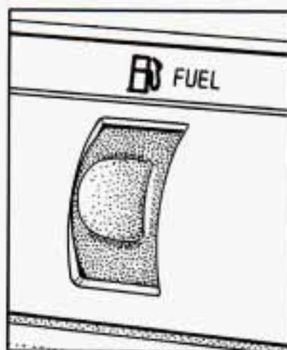
To open the fuel door (on the left of the vehicle), press the button next to the trunk release button, to the right of the steering column. The ignition does not need to be on. The remote fuel door release will work in all transaxle positions.
