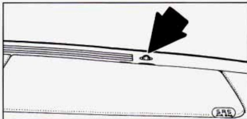
Your automatic electronic climate control system has two sun sensors located on the top of the instrument panel that detect direct sunlight. To keep you and your passengers comfortable, the system may supply cooler air to the side toward the sun. Be careful not to put anything over these sun sensors. The automatic electronic climate control system may not operate correctly if these sensors are covered.
