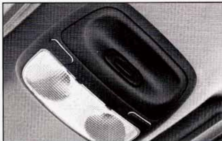
This transmitter allows you to consolidate the functions of up to three individual hand-held transmitters. It will operate garage doors and gates, or other devices controlled by radio frequency such as home and office lighting systems.
