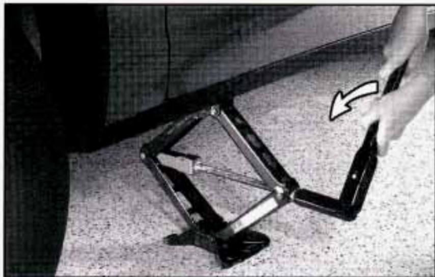
10. Lower the vehicle by rotating the wheel wrench counterclockwise on the jack. Lower the jack completely.
