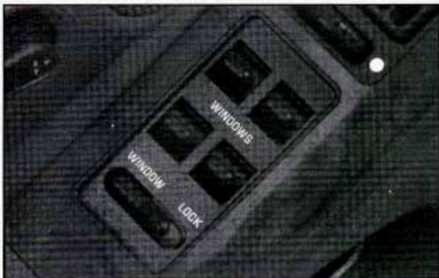
Switches on the driver's armrest control each of the windows while the ignition is on or Retained Accessory Power is active. In addition, each passenger's door armrest has a switch for its own window.
