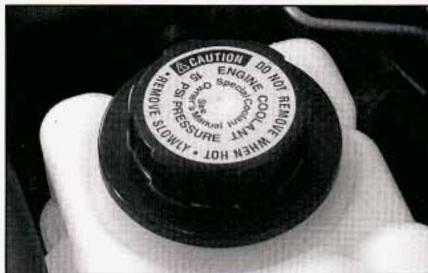
The engine coolant surge tank is located on the driver's side of the engine compartment.
