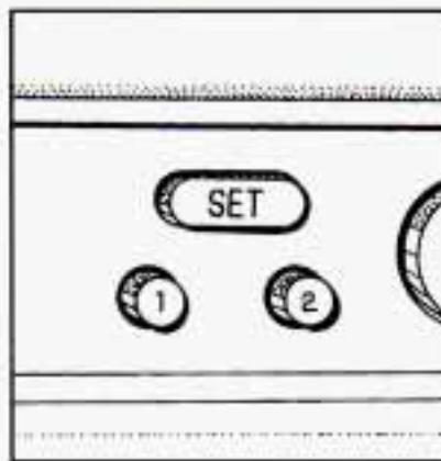
The memory function controls both the driver's seat and outside mirror positions. To set your memory seat and mirrors:
