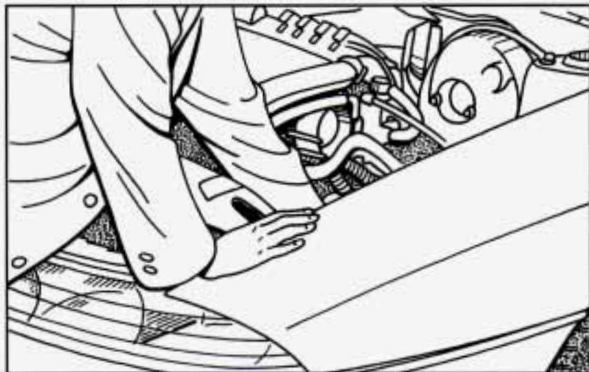
2. Twist the bulb assembly one-sixth of a turn counterclockwise and pull out the bulb assembly.
