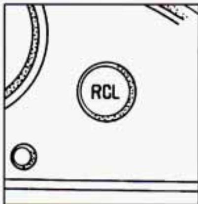
When you press the RCL button, the system scrolls through any currently active warning messages, then returns to the mode the system was in before you pressed RCL.
