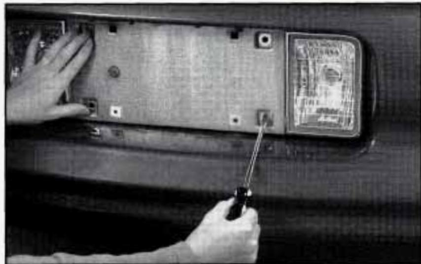
3. Pry off the cover and pull down to access the bulbs.
