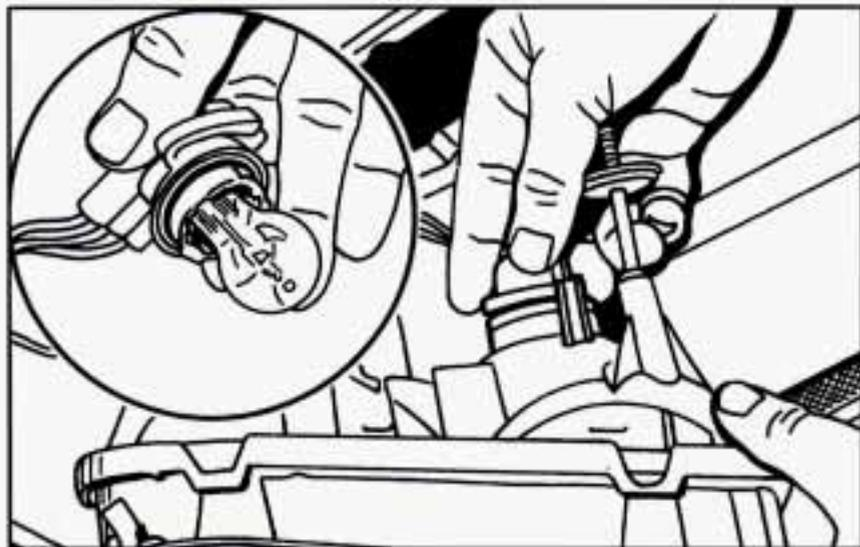
5. Pull out the taillamp assembly to reach the bulb and pull it out. To replace, push the bulb back in.
