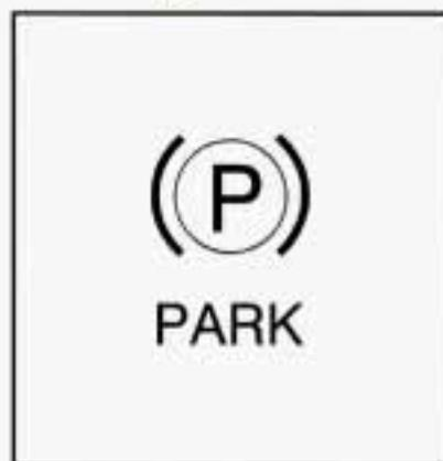
When the ignition is on, this light will come on when you set your parking brake. The light will stay on if your parking brake doesn't release fully. If you try to drive off with the parking brake set, a chime will also come on until you release the parking brake.
