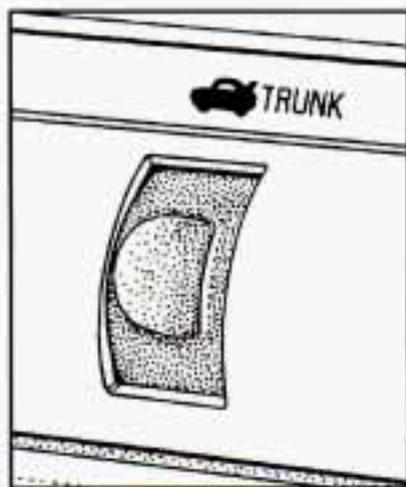
Press the TRUNK release button located to the right of the steering column to release the trunk lid. The trunk release override switch must be in the on position.
