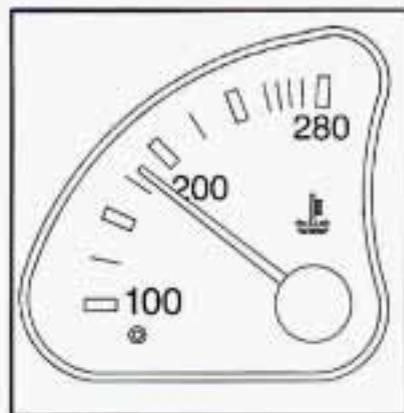
This gage shows the engine coolant temperature.
