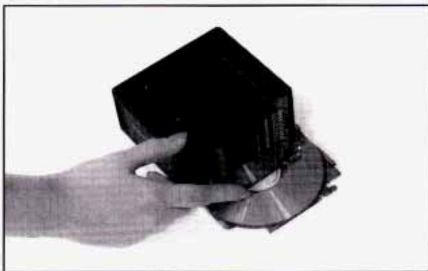
You must first load the magazine with discs before you can play a compact disc. Each of the 12 trays holds one disc. Press the button on the back of the magazine and pull gently on one of the trays. Load the trays from bottom to top, placing a disc on the tray with the label
