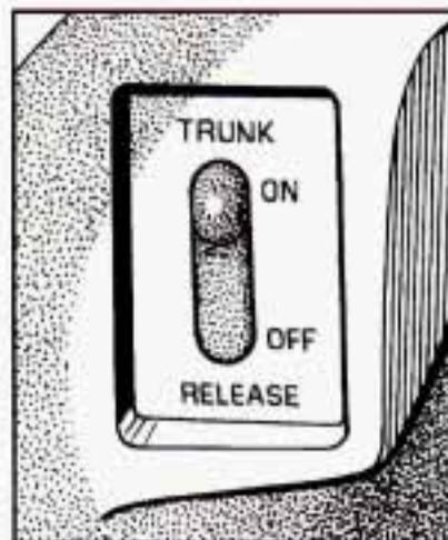
The trunk release switch in the glove box allows you to secure items in the trunk.
