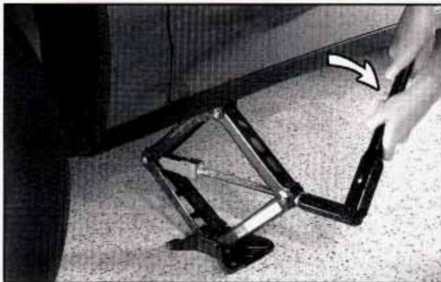
5. Raise the vehicle by rotating the wheel wrench clockwise in the jack. Raise the vehicle far enough off the ground so there's enough room for the spare tire to fit.
