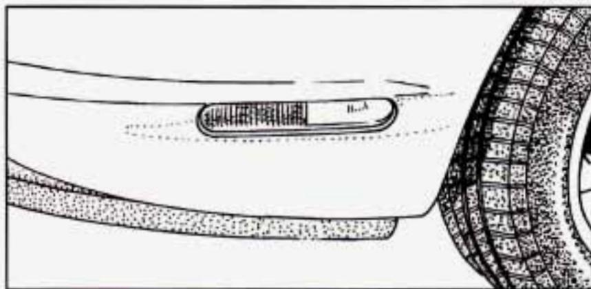
The cornering lamps are designed to come on when you signal a turn. This will provide more light for cornering at night.
