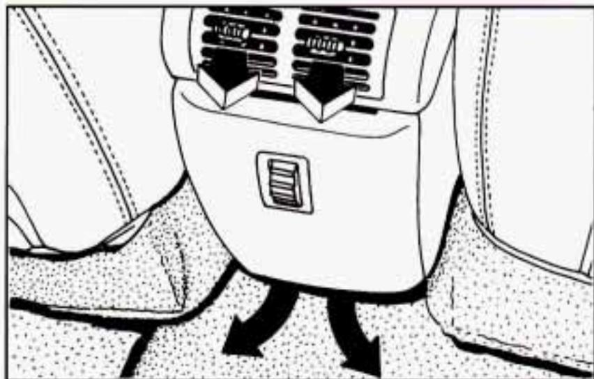
Rotate the control between the rear outlets up to direct air through the upper outlets. Rotate the control down to direct air through the lower outlets. Adjust the direction of airflow from side to side with the controls in each outlet.
