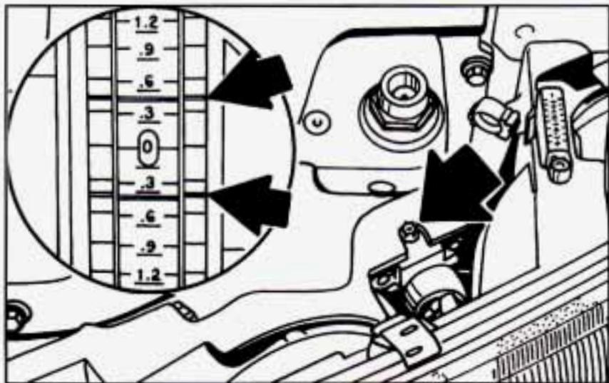
1. Check the vertical aim for each headlamp. The vehicle must be on a level surface. Turn the vertical aiming screw until the bubble in the level is centered at 0 (zero).
