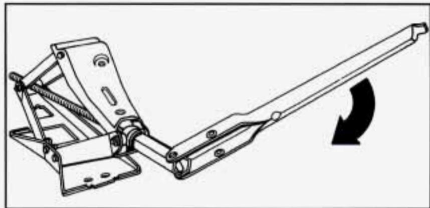
3. Turn the wheel wrench clockwise by hand to raise the jack head a few inches.
