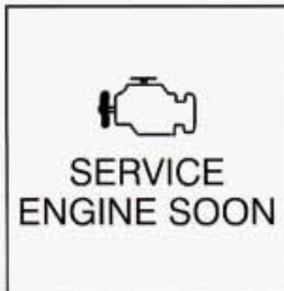
Your Aurora is equipped with a computer which monitors operation of the fuel, ignition and emission control systems.
