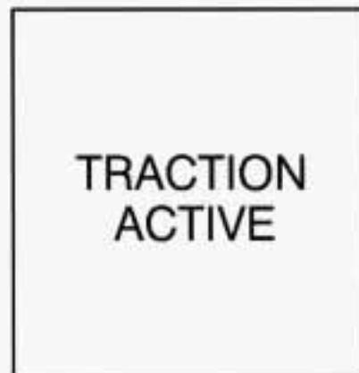
This light will come on when your traction control system is limiting wheel spin. See "Traction Control System Active Light" in the Index.
