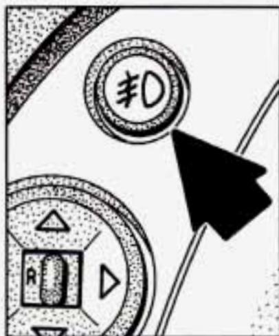
To turn on the fog lamps, first turn on the parking lamps or headlamps. Then press the fog lamp switch located on the left side of the instrument panel. A light will glow on the switch when the switch is on. To turn off the fog lamps, press it again.
