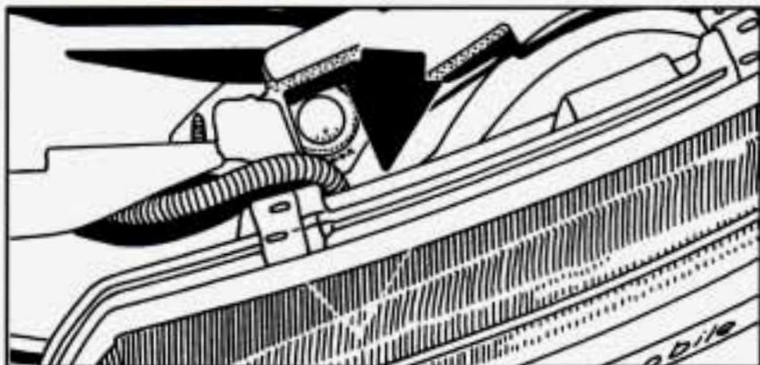
3. Now you can reach in behind the lamp housing and pull out the bulb.
