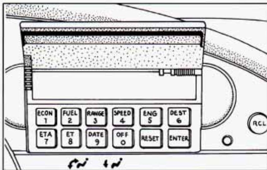
The Driver Information Center (DIC) displays information in either English or metric. When the system is on or off, push the OFF button down for two seconds to change the display between English and metric. This will also change the digital screen for the climate control system between English and metric.
