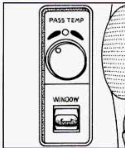
With this feature, the right front seat passenger can control the comfort setting for their own zone. To use this feature, adjust the control on the passenger's side armrest to the desired comfort level.
